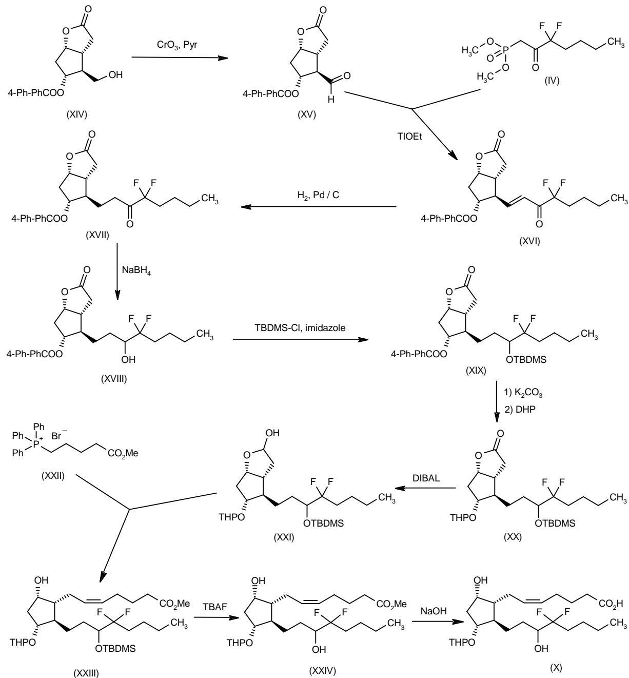
Hydrolysis of the ester group of compound (XIX) in basic medium, followed by reaction with dihydropyran yields the tetrahydropyranyl ether (XX), which is reduced with DIBAL to afford the lactol (XXI). Condensation of lactol (XXI) with 4-(methoxycarbonyl)butyl triphenylphosphonium bromide (XXII) provides the unsaturated methyl ester (XXIII), which is desilylated by means of TBAF in THF to
